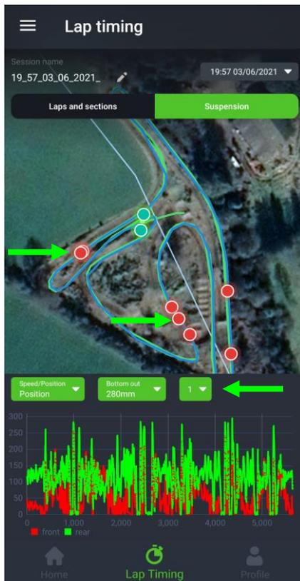
Red circles will appear on the track where the front and / or rear suspension has been compressed by **more** than the mm value you have typed in. In this example, the red circles show where the front and / or rear suspension has been compressed by more than 280mm.
